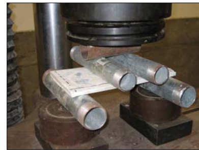
Figure 3: Tile Plate Testing
