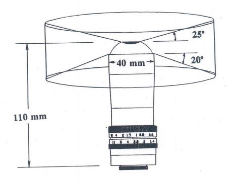
**Figure 2.** A 38 mm diameter PAL imaging system. Figure courtesy of Optechnology, Inc., Gurley, AL.
