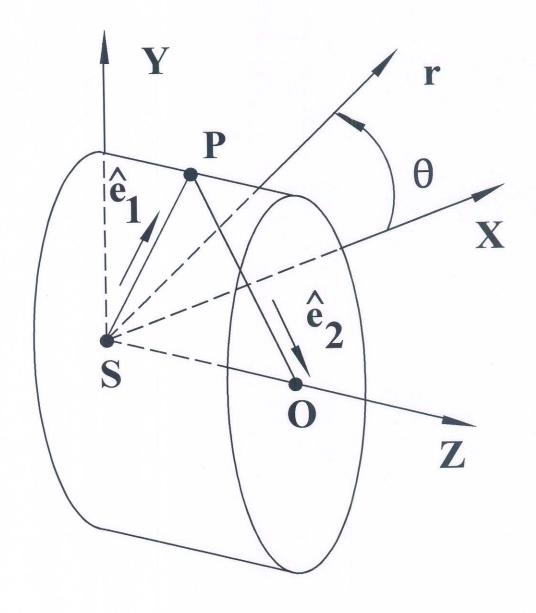
Figure 3. Cartesian (x,y,z) and cylindrical  $(r,\theta,z)$  systems used to describe object space.
