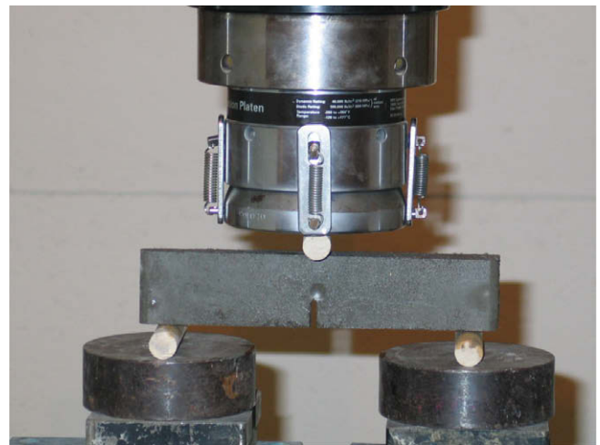
Fig. 7. Three points bending apparatus for testing single edge notch bend (SENB) specimens.
