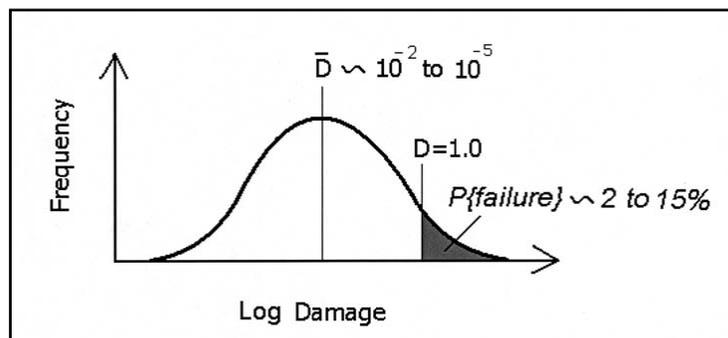
**Figure 3.** Failure probability distribution due to cumulative damage.
