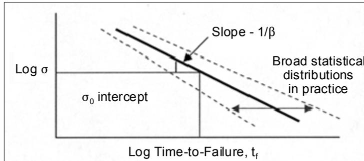
**Figure 2.** Time-to-failure versus damage due to increased stress.
